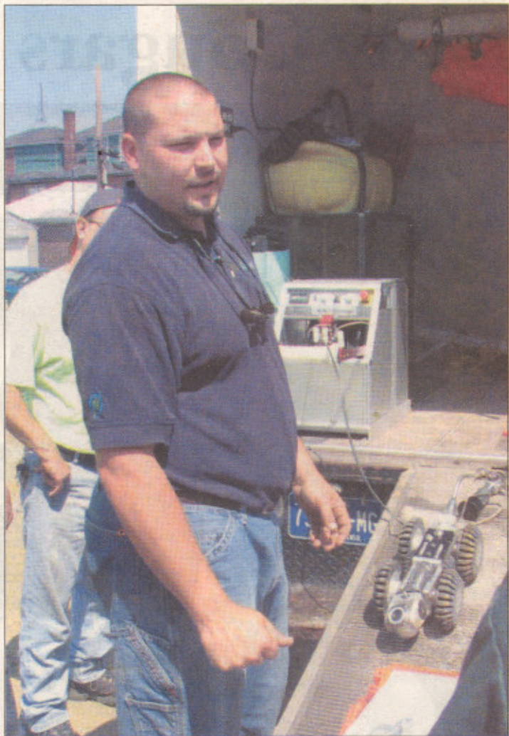
Mike Vislay of EnviroSight , Randolph, N.J., is the manufacturer of a sewer camera, right, that looks like a little car. The camera is mounted at the front of the 14½-inch body that allows the camera to be maneuvered within sewer or water lines. Mountain Council of Governments and six area governmental entities shared in its cost and will share in its use in sewer lines. 103/06
